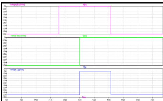
Fig. 4. Write operation of CMOS SRAM
