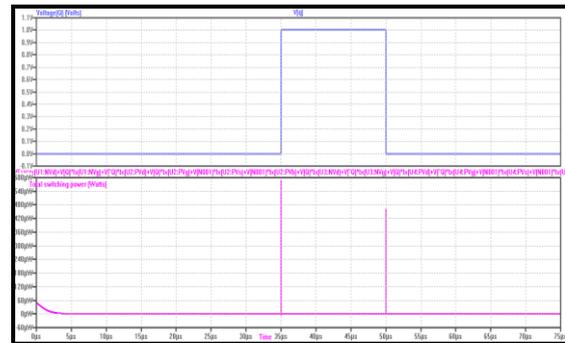
Fig. 6. Total switching power in CMOS SRAM during write operation
