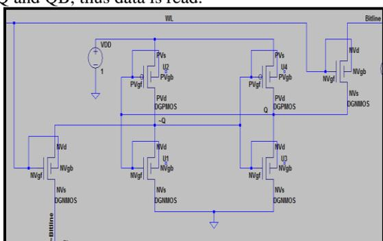
Fig. 1. 6T SRAM cell using FinFET
