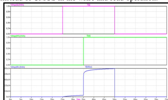
Fig. 8. Read operation of CMOS SRAM
