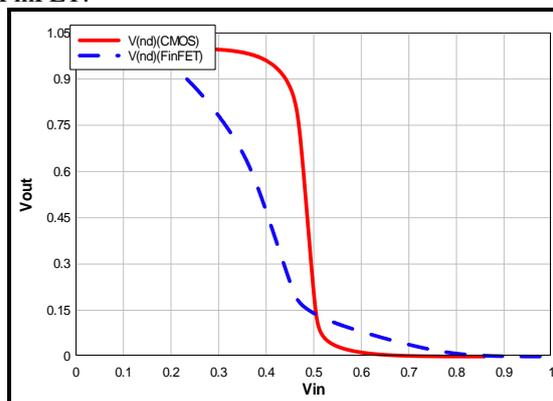
Fig. 2. Voltage transfer characteristics of FinFET and CMOS at 45 nm node
