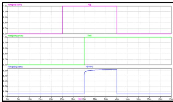
Fig. 9. Read operation of FinFET SRAM
