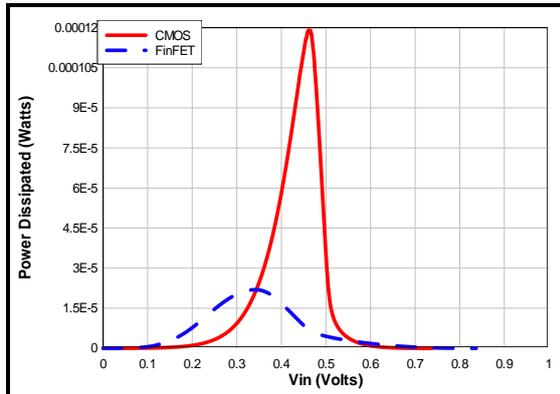
Fig. 3. Power dissipation of NMOS in FinFET and CMOS inverters at 45 nm node
