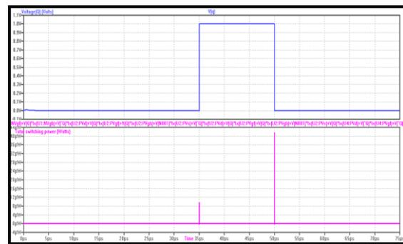
Fig. 7. Total switching power in FinFET SRAM during write operation
